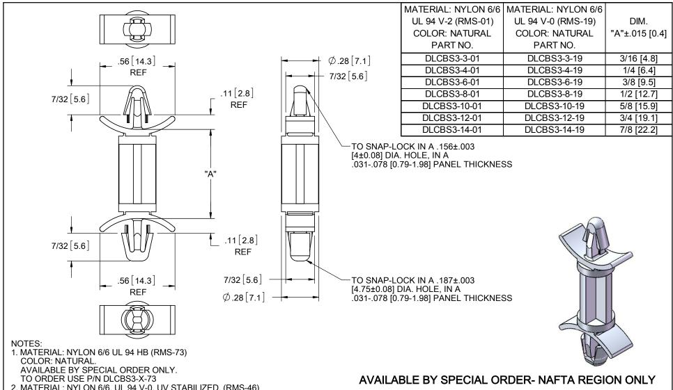
2. MATERIAL: NYLON 6/6, UL 94 V-0, UV STABILIZED, (RMS-46)
